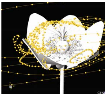
Particle tracking functionality used to simulate the fertilization of kiwifruit by blowing pre-collected pollen onto the flowers
