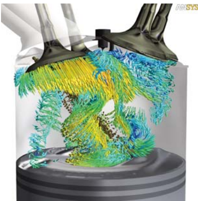
Vortex structures in a four-stroke engine just after injection of fuel and intake valve opening Courtesy of BMW Group
